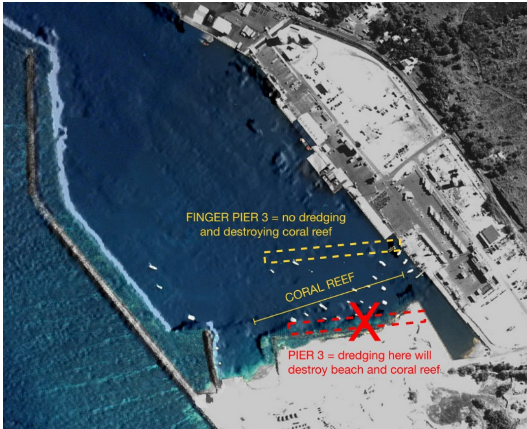
Proposed relocation of future Pier 3 to protect the coral reef. This location requires minimal dredging and will satisfy coral reef protection per EO 13089
